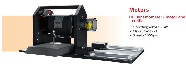
The aluminium cradle which houses our dynamometer features a rugged and safe sliding mechanism into which each of the other six motors in the range fix into position. The motor coupling meets the dynamometer in a protected housing and allows for safe study of each machine type at 24 volts. When using our system in manual mode, it is likely you will require two (per set) HP1324 Fluke 115 True RMS Digital Multimeter and one HP8067 Tektronix Digital oscilloscope.
