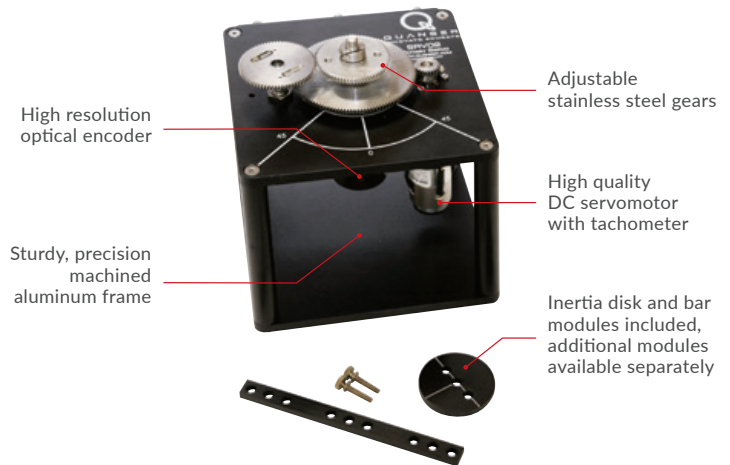
Rotary Servo Base Unit with Inertia Loads
