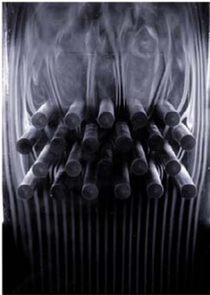
SMOKE TRAILS AROUND THE HEAT EXCHANGER MODEL FROM THE AF80B SET
