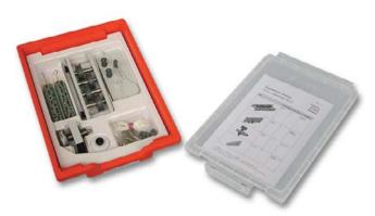
Students fit the parts to the work panel and apply effort and load weights to find their relative mechanical advantage and efficiency.
