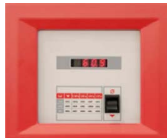
ONE-BUTTON OPERATION EQUIPMENT FOR STANDARDISED ROCKWELL MEASURING
